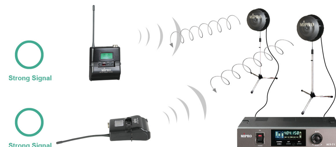
Figure 3: How the signal quality present between the linear and the circular polarization antennas
