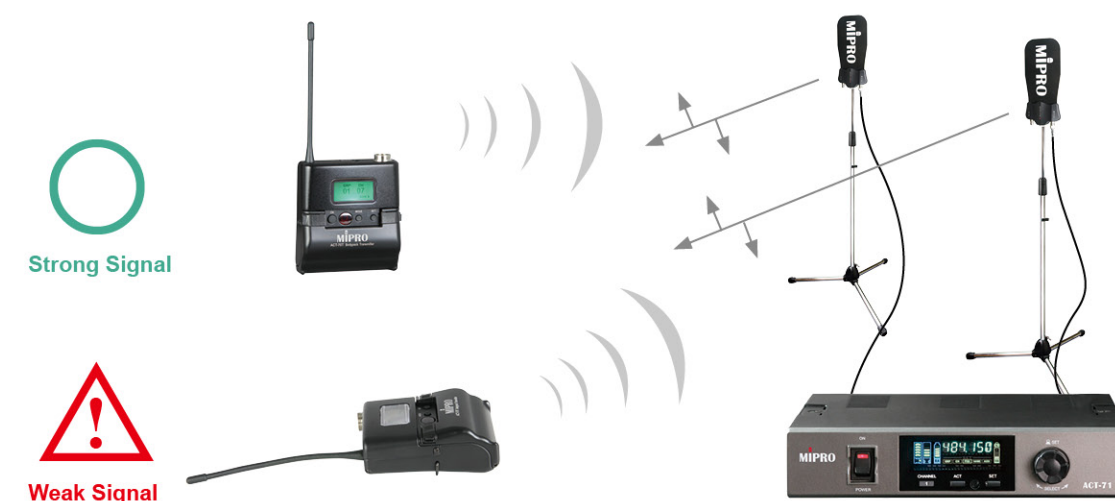
Figure 2: How the signal quality present between the linearly polarized antennas
