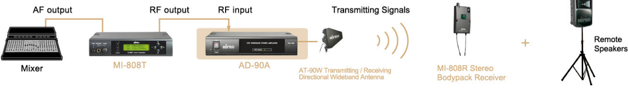
Application of AD-90S with MI-808T Stereo Transmitter & AT-90W Transmitting / Receiving Directional Wideband Antenna
